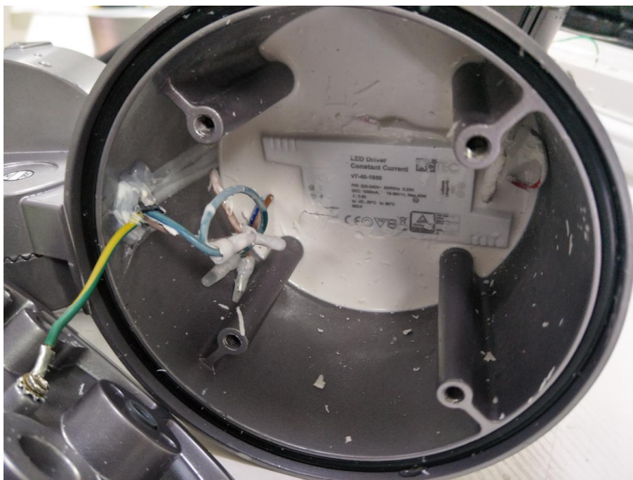
Photo 4: Test result after IP6X and IPX6 test
