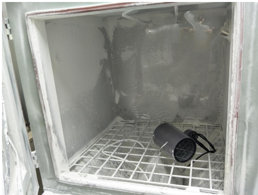
Photo 2: IP6X test of model BL-D150-1204A
