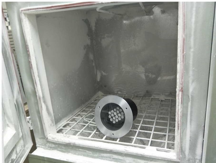
Photo 2: IP6X test of model BL-BDA1802
