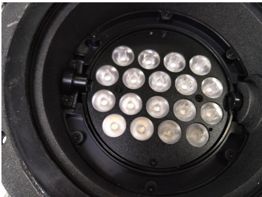
Photo 4: Test result after IP6X and IPX7 test
