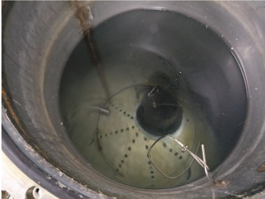
Photo 3: IPX7 test of model BL-BDA1802
